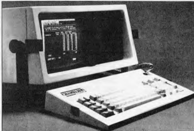
The Chameleon micro, weighing 28lb, is marketed by Seequa as a low-cost IBM running 8-bit CP/M software.
