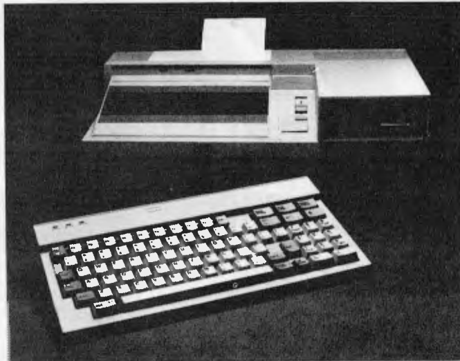
The STM portable personal computer weighs less than 17lb and includes 256k of RAM (expandable to 512k).
